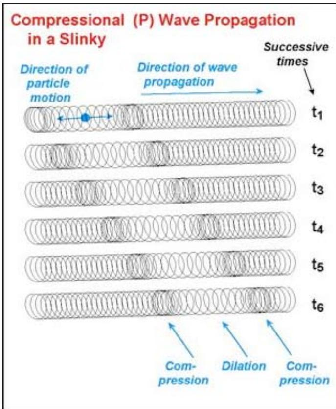
Compressional (P) wave propagation in a slinky. A disturbance at one end results in a compression of the coils followed by dilation (extension), and then another compression. With time (successive times are shown by the diagrams of the slinky at times  $t_1$  through  $t_6$ ), the disturbance propagates along the slinky. After the energy passes, the coils of the slinky return to their original, undisturbed position. The direction of particle motion is in the direction of propagation.
