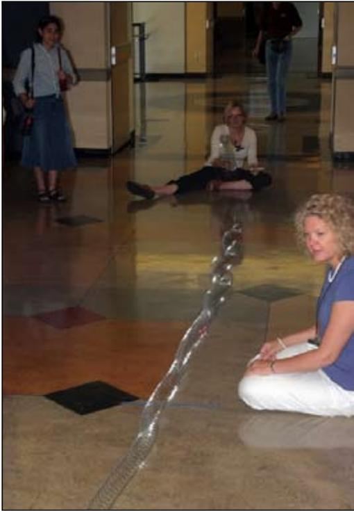
Master Teacher Bonnie Magura demonstrates S waves using two metal slinkies taped together. Attach a small paper “flag” to the taped joint to emphasize the movement directions.
